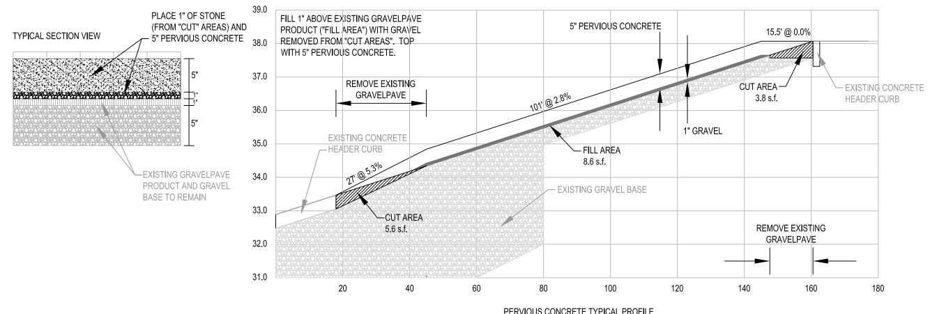
PERVIOUS CONCRETE TYPICAL PROFILE
